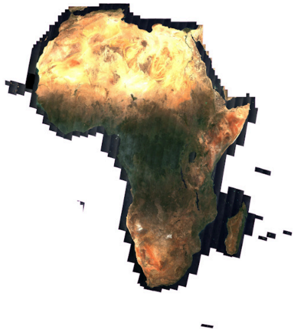
Image: A cloud-free image of all of Africa produced by combining tens of thousands of satellite image collected throughout an entire year
